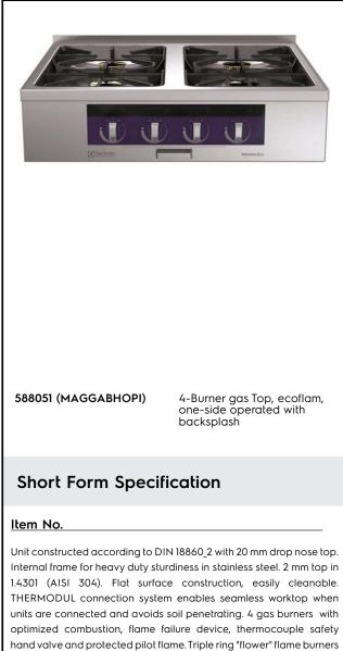
with anti-clogging design. Manual gas valves allow precise flame intensity control. Large pan support in cast iron with long center fins for various pan sizes. ECOFLAM pan detection system to save energy and to reduce unnecessary heat radiation in the kitchen. Deep flat spillage tray with rounded corners and drain hole. Metal knobs with embedded hygienic silicon "soft" grip enable easier handling and cleaning.
